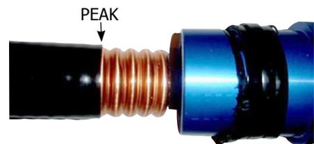
4. Install O-ring in the valley next to the jacket cut. Apply grease as per connector instructions.
