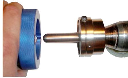
7. Using drill turning clockwise on low RPM to cut the end of the cable with the Trim Head.
